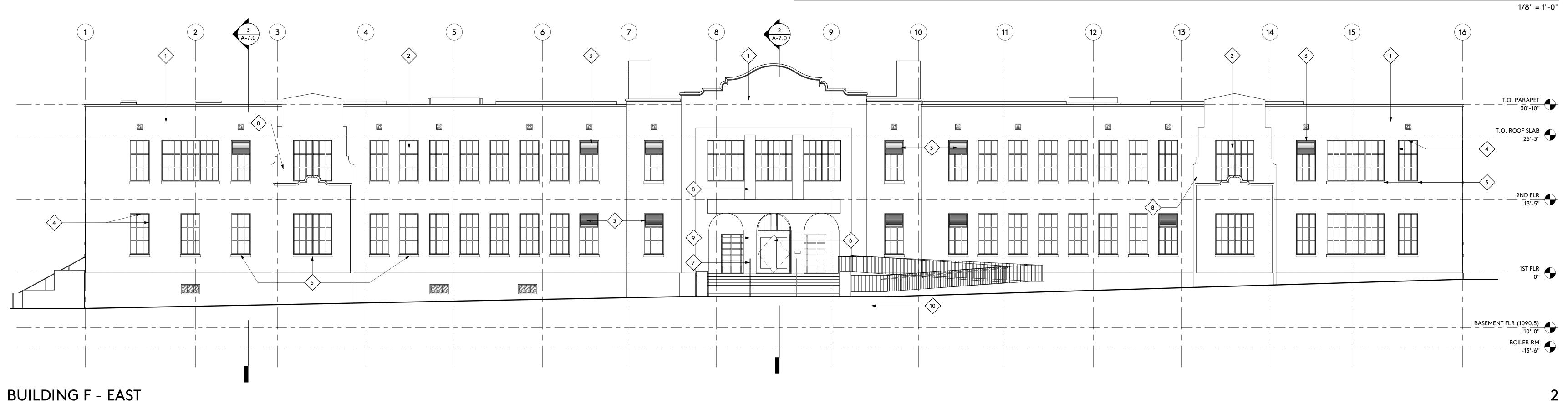
EXISTING SMOOTH EXTERIOR CEMENT PLASTER WALLS TO REMAIN. REPAIR ALL WALLS DAMAGED DUE TO MODERNIZATION. RESTORE SURFACES AS REQUIRED TO MAINTAIN SAME APPEARANCE THROUGHOUT.
