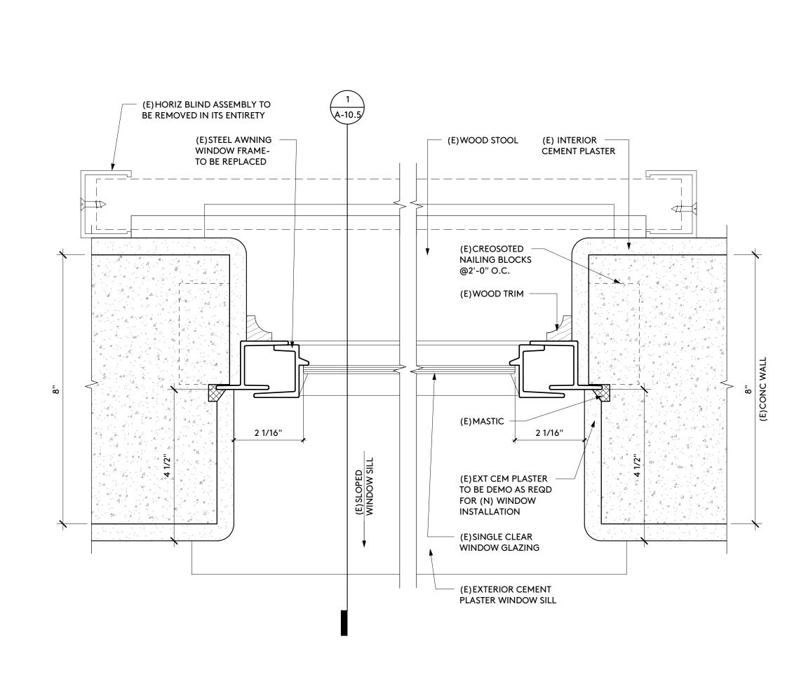
BASIS OF DESIGN: ARCADIA - INTEGRA SERIES MW-40 FIXED STEEL WINDOWS STEEL WINDOW JAMB @ SHOTCRETE SHEAR WALL
