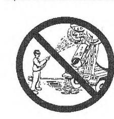
✓ Divert water from washing exposed aggregate concrete to a dirt area where it will not run into a gutter, street, or storm drain.
