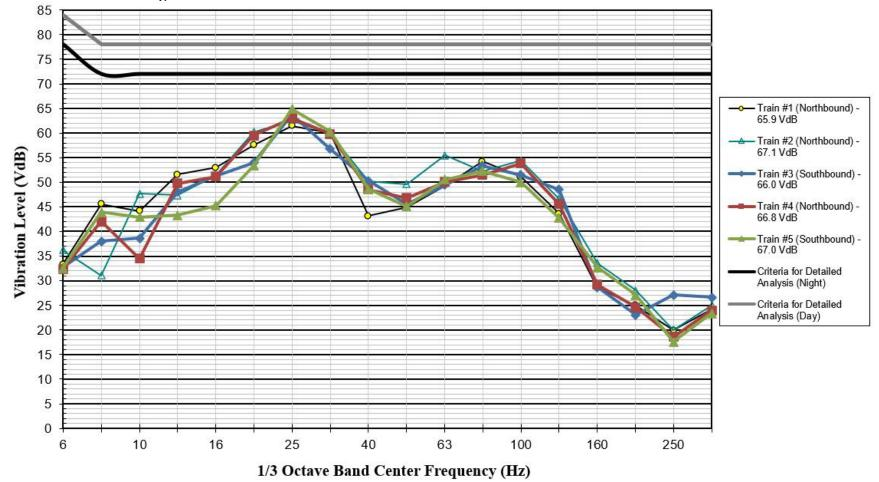
FIGURE A7 VTA Light Rail Train Vibration Levels at V-1
