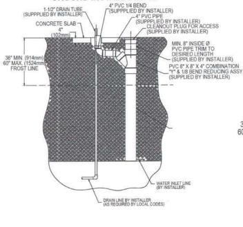
( Ø 14" (356mm) 29" (737mm) Ø 10' (254mm) 14-9/16" (371mm) SEE DETAIL A 0 44" 33-7/16" (1118mm) 19" (850mm) (483mm) B-30" 27-1/8" (762mm) (689mm) (203mm) **DETAIL A** (102mm) AIR GAP / VACUUM BREAKER 1-1/4" DRAIN TUBE SUPPLIED WITH FTN AIR GAP ASSY 36" MIN. (914mm) 60" MAX. (1524mm) FROST LINE SUPPLIED WITH VALVE 1-1/2" DRAIN TUBE SUPPLIED BY ñ WATER INLET LINE (BY INSTALLER) VALVE WATER LINE SUPPLIED WITH A 1/4 X 1/2 NPT CONNECTOR DRAIN LINE BY INSTALLER
