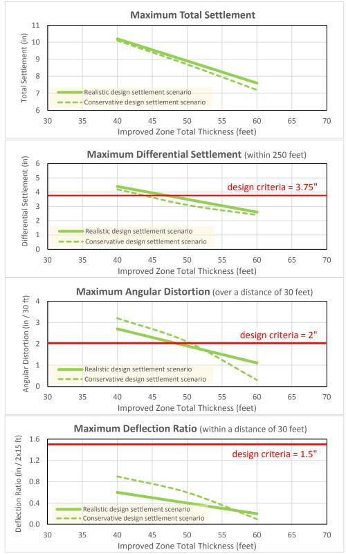
Figure 1. Design settlement parameters for Typical Design Case (Scenario 1)
