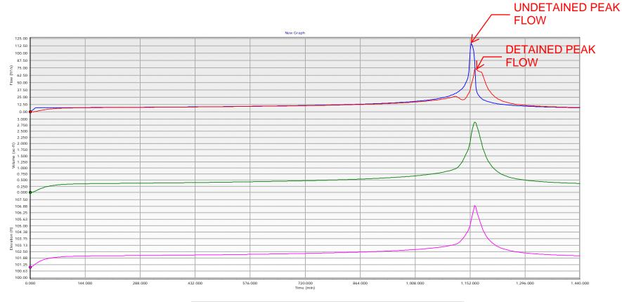
PO-1 - Base - Flow (Total In) - PO-1 - Base - Flow (Total Out) - PO-1 - Base - Volume - PO-1 - Base - Elevation
