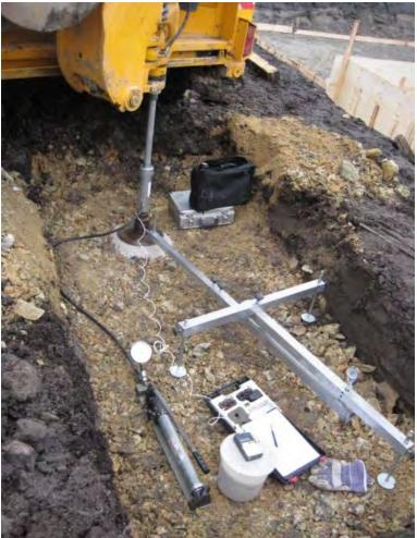
Figure 2. Plate load test configuration.
