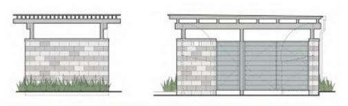
EAST & SOUTH ELEVATIONS - WASTE TRANSFER ENCLOSURE
