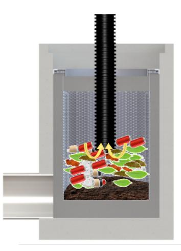
Insert the vacuum hose down into the filter basket and suck out debris. Use a pressure washer to assist in vacuum removal. Pressure wash off screens.
