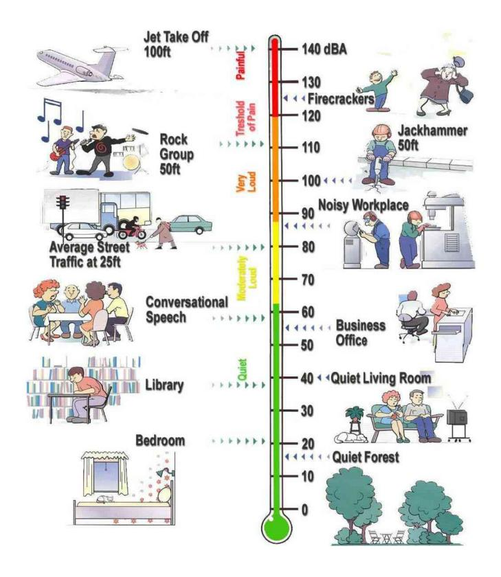
Figure 3 Weighted Sound Levels and Human Response
