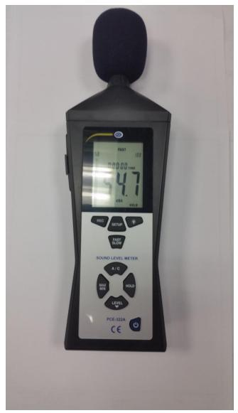
Figure 3: PCE-322A noise meter used in study
