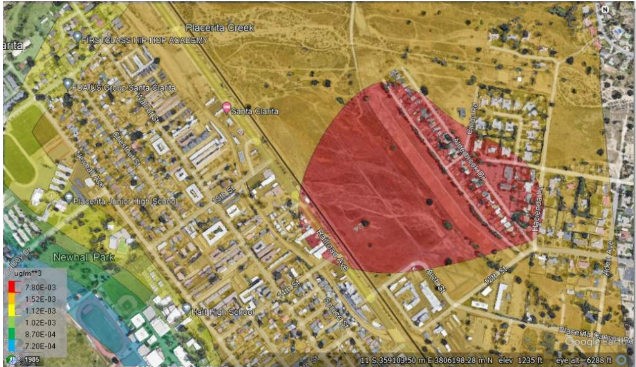
Figure 4: DPM Concentrations From Generators On Site
