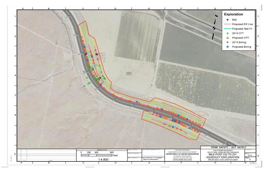
Figure 2. Geotechnical Exploration Methods and Location Centered at Milepost 230.75 and 231.3
