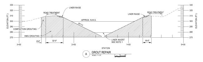
Figure 4. Cross Section of Embankment with Grouting Alternative
