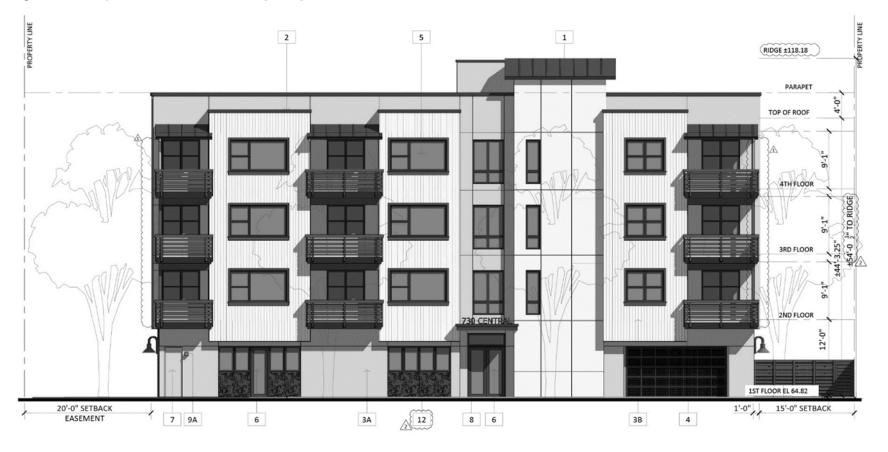
Figure 3 Proposed Central Avenue (Front) Elevation
