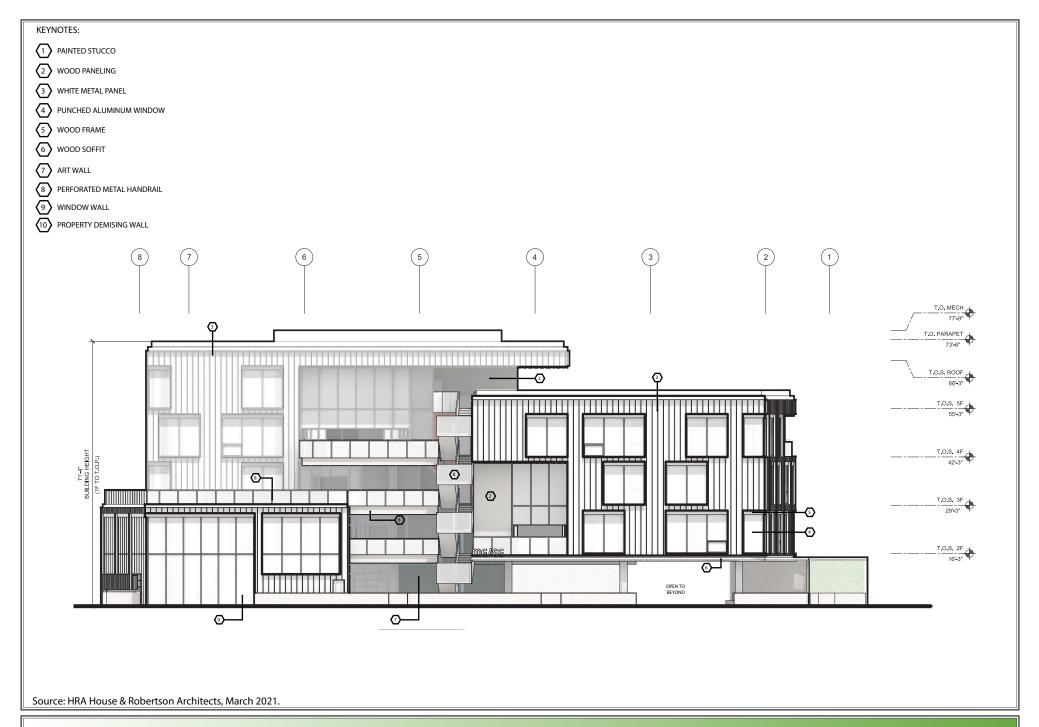
Figure 3.12 East Elevation
