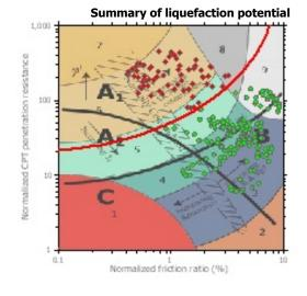
Zone A<sub>1</sub>: Cyclic liquefaction likely depending on size and duration of cyclic loading Zone A<sub>2</sub>: Cyclic liquefaction and strength loss likely depending on loading and ground geometry
