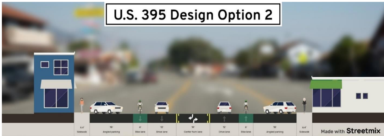
Figure 1-3: Design option 2 (showing a three-lane configuration, dedicated bike lanes, back-in diagonal parking and sidewalks).
