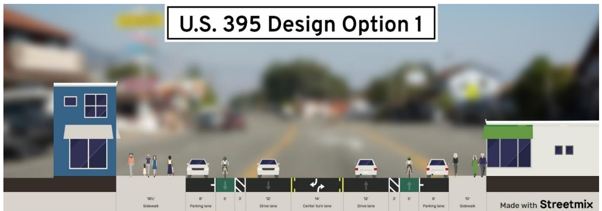
Figure 1-2: Design option 1 (showing a three-lane configuration, dedicated, buffered bike lanes, parallel parking and sidewalks).
