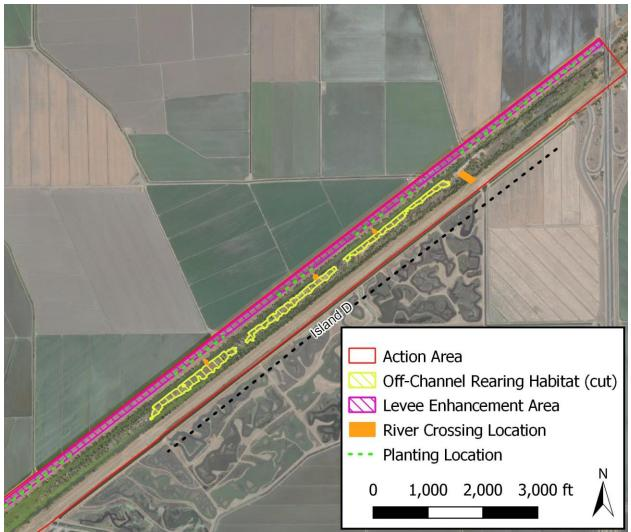
Figure 3. Project conceptual design for the upstream portion of the Project site with grading for off-channel habitat and levee enhancement areas as indicated.
