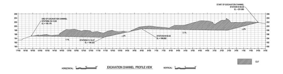
**Figure 11 Channel Excavation Sections**
