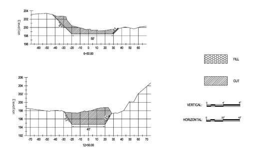
EXCAVATION CHANNEL CROSS SECTIONS
