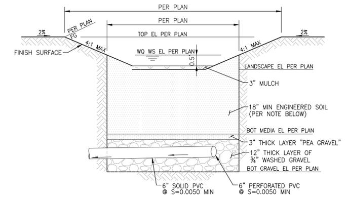
BIORETENTION FACILITY DETAIL (TYP)
