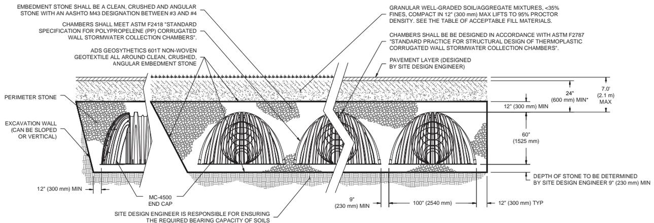
\*MINIMUM COVER TO BOTTOM OF FLEXIBLE PAVEMENT. FOR UNPAVED INSTALLATIONS WHERE RUTTING FROM VEHICLES MAY OCCUR, INCREASE COVER TO 30" (750 mm).
