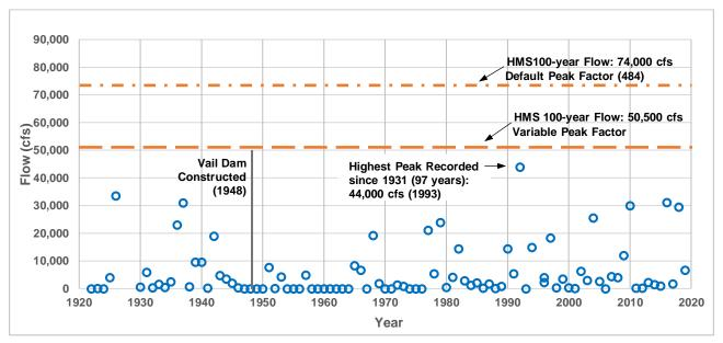
Figure 4.7. Santa Margarita River Peak Flow Comparison at Ysidora USGS Gage
