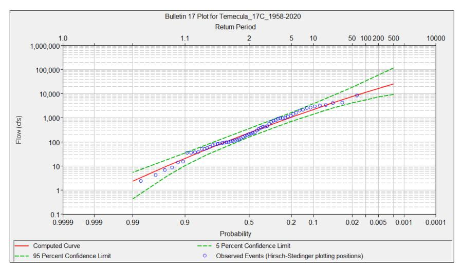
Figure A-2. Temecula Creek near Aguanga Flood-Frequency Curves from HEC-SSP (USGS gage #11042400)
