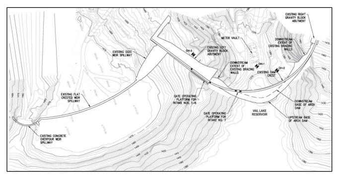
Figure 3.5. Vail Lake Existing Dam and Spillway (LSA, 2020)
