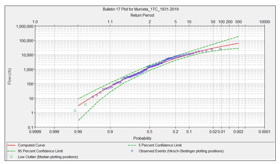
Figure A-3. Murrieta Creek near Temecula Flood-Frequency Curves from HEC-SSP (USGS gage #11043000)
