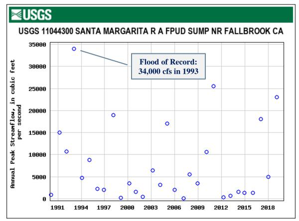
Figure 2.2. Annual Peak Streamflow at USGS Gage #11044300 (Santa Margarita River near Fallbrook)
