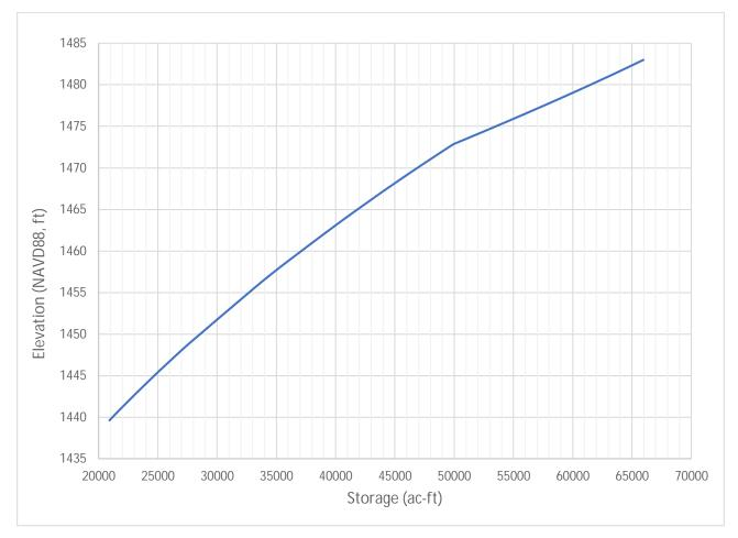
Figure 3.4. Vail Lake Elevation-Storage Curve
