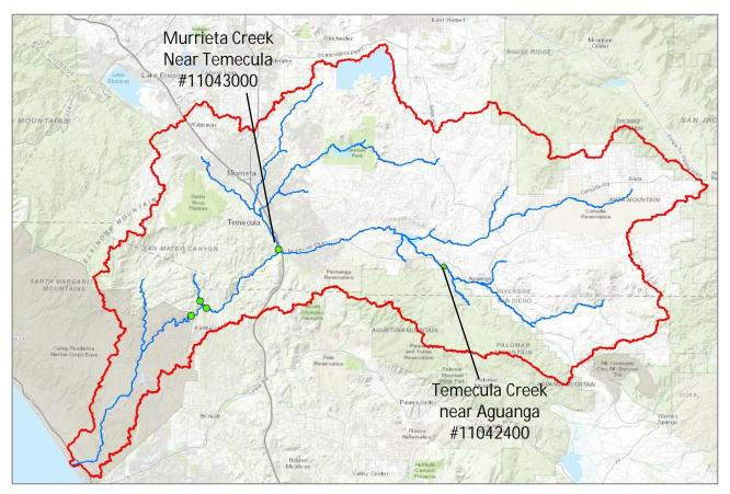
Figure A-1. USGS Streamgage Locations used in the Flood Frequency Analysis
