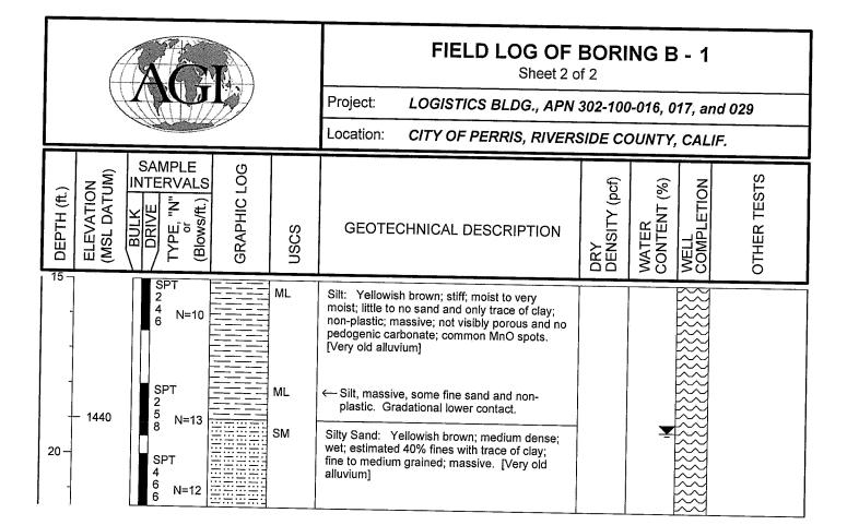
Bottom of boring at 21.5 ft. Perched groundwater encountered at 19.2 ft. Boring backfilled with compacted soil cuttings.
