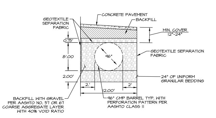
CMP DETENTION SYSTEM TYPICAL DETAIL
