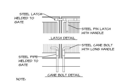
TRASH ENCLOSURE GATE LATCHES DETAIL
