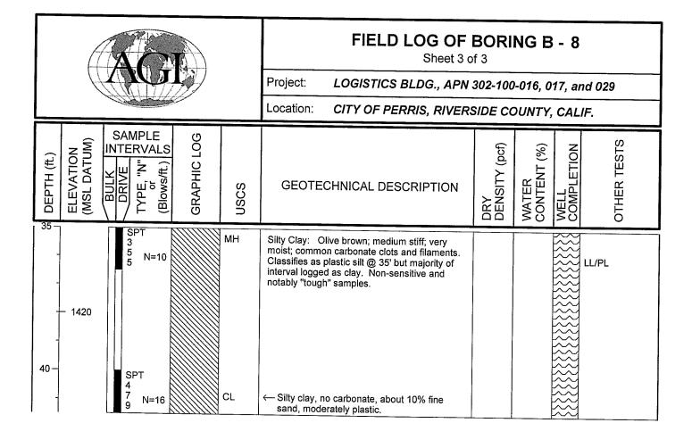
Bottom of boring at 41.5 ft. Groundwater measured at 20.0 ft. Boring backfilled with compacted soil cuttings.
