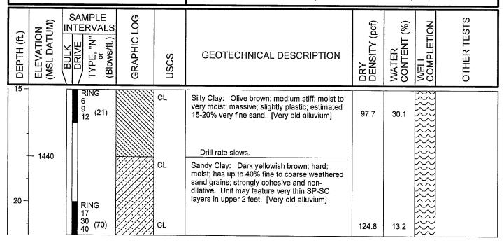
Bottom of boring at 21.5 ft. No groundwater measured. Boring backfilled with compacted soil cuttings.
