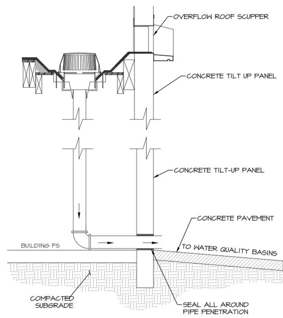
**ROOF DRAIN DETAIL**
