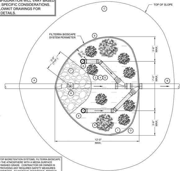
AS WITH ALL OPEN TOP BIOTENTION SYSTEMS, FILTERRA BIOSCAPE SYSTEM IS OPEN TO THE ATMOSPHERE WITH A MEDIA SURFACE RECESSED BELOW FINISHED GRADE. CONTRACTOR OR OWNER IS RESPONSIBLE FOR PROVIDING ANY REQUIRED SAFETY MEASURES AROUND SYSTEM PERIMETER. TO MAINTAIN AESTHETICS, REMOVAL OF HEAVY STORMWATER DEBRIS MAY BE NECESSARY BETWEEN REGULAR FILTERRA SYSTEM MAINTENANCE EVENTS.
