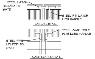
**TRASH ENCLOSURE GATE LATCHES DETAIL**
