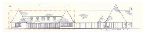
Figure 48: Plan east elevation (labeled south in the drawings) of the Main Lodge as recorded in 1983, not long after UCLA took control of the site. Original part of the lodge in dashed outline. Source: A-3, Exterior Elevations, Existing Lodge Record Drawings, Cashion, Horle, Cocke, Gonzalez Architects, May 26, 1983.
