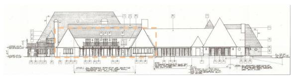
Figure 49: Plan east elevation of the Main Lodge with the proposed 1984 addition to the rear. Original part of the lodge in dashed outline. Source: ML-6, Exterior Elevations, Main Lodge and Rose Relocation, Leidenfrost/Horowitz & Associates, August 2, 1984.
