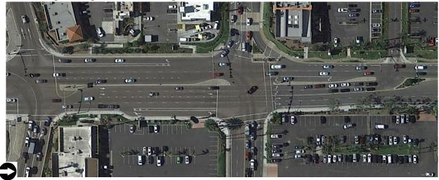
**Montiel Road**, between Nordahl Road and Leora Lane, is unclassified in the *City of San Marcos General Plan Mobility Element*. It is currently constructed as a 2 lane undivided roadway with a two-way left-turn lane. The posted speed limit is 40 mph.
