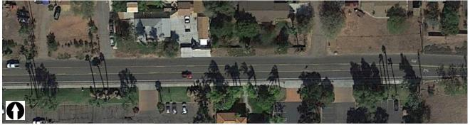
**Montiel Road**, between Leora Lane and Rock Springs Road, is unclassified in the *City of San Marcos General Plan Mobility Element*. It is constructed as a 2 lane undivided roadway. The posted speed limit is 40 mph, and on-street parking is permitted.
