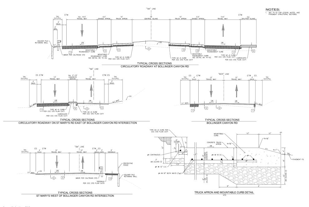
Figure 2.2-2b: Proposed Roundabout Sections
