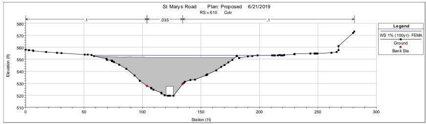
Figure 8. Upstream Face of the Cross Culvert under Proposed Condition, Looking Downstream
