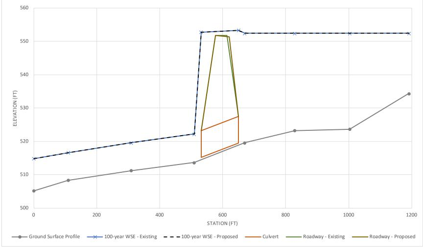
Figure 9. 100-year Flood Profile, Existing and Proposed Conditions
