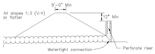
EMBANKMENT SECTION THRU RISER
