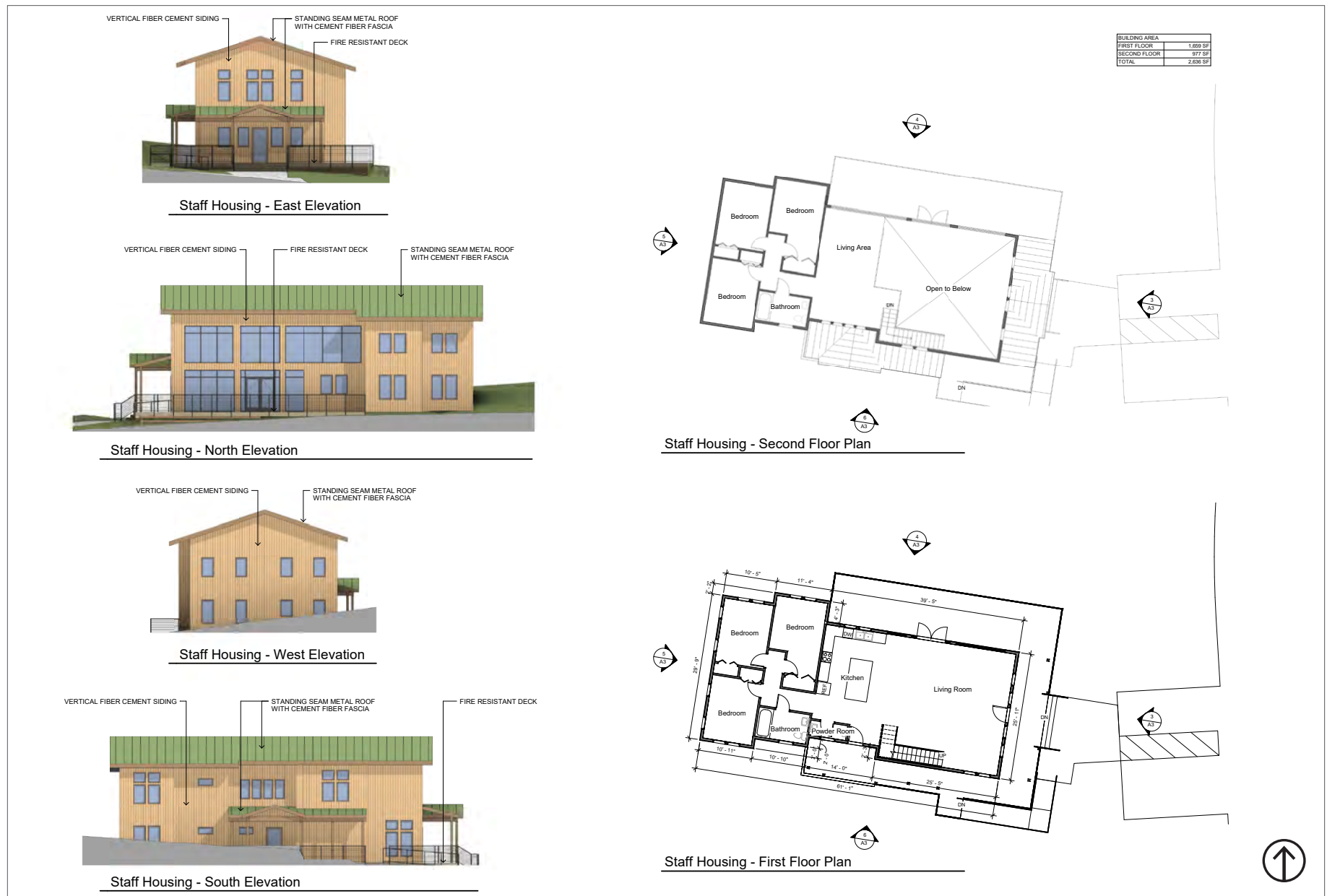
Figure 3-11 Staff Housing - Floor Plans and Elevations
