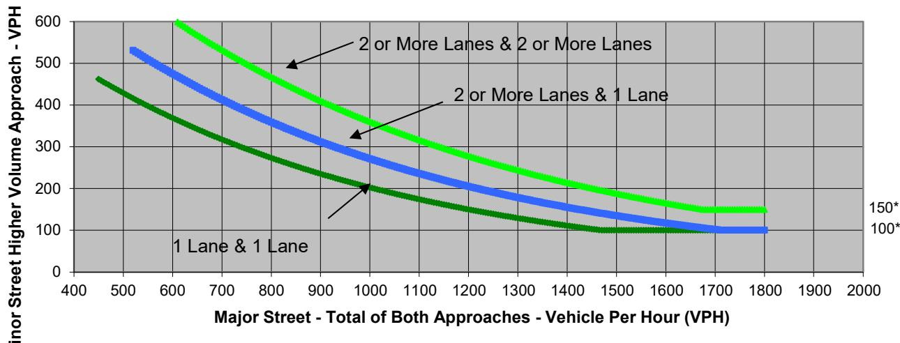
\* Note: 150 vph applies as the lower threshold volume for a minor-street approach with two or more lanes and 100 vph applies as the lower threshold volume for a minor-street approach with one lane.
