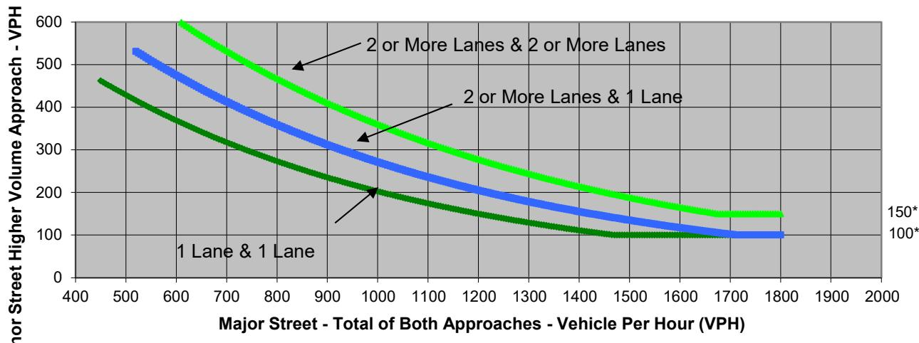
\* Note: 150 vph applies as the lower threshold volume for a minor-street approach with two or more lanes and 100 vph applies as the lower threshold volume for a minor-street approach with one lane.
