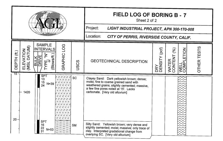
Bottom of boring at 21.5 ft. No groundwater encountered. Boring backfilled with compacted soil cuttings.
