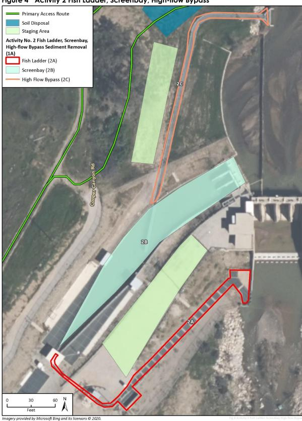
Figure 4 Activity 2 Fish Ladder, Screenbay, High-flow Bypass
