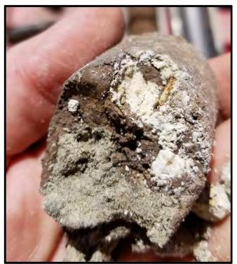
Figure 4-2. Undocumented Artificial Fill-Silty to Clayey Sand.
