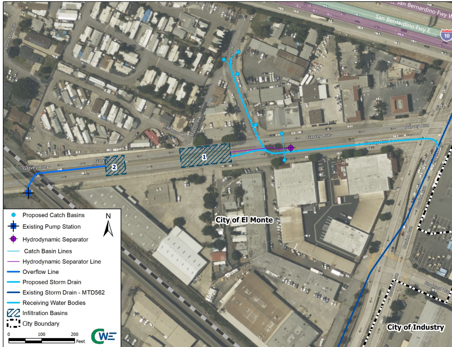
Figure 2-2 Proposed Storm Drain Alignment and Infiltration Gallery
