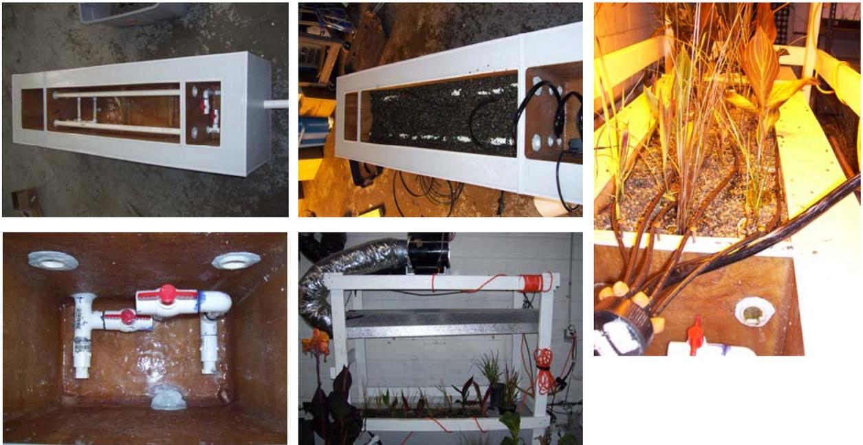
Specifications of the model are as follows (inside dimensions): 5.5 ft. in length, 1 ft. wide and 1 ft. tall. All internal piping was also sized to scale. The model was then water tested to ensure no leaks between chambers or piping joints. The sub surface flow wetland chamber was filled with a specific mixture of pre-washed 3-5mm pea gravel and BioMediaGREEN. The wetland chamber was then planted with various wetland plants.
