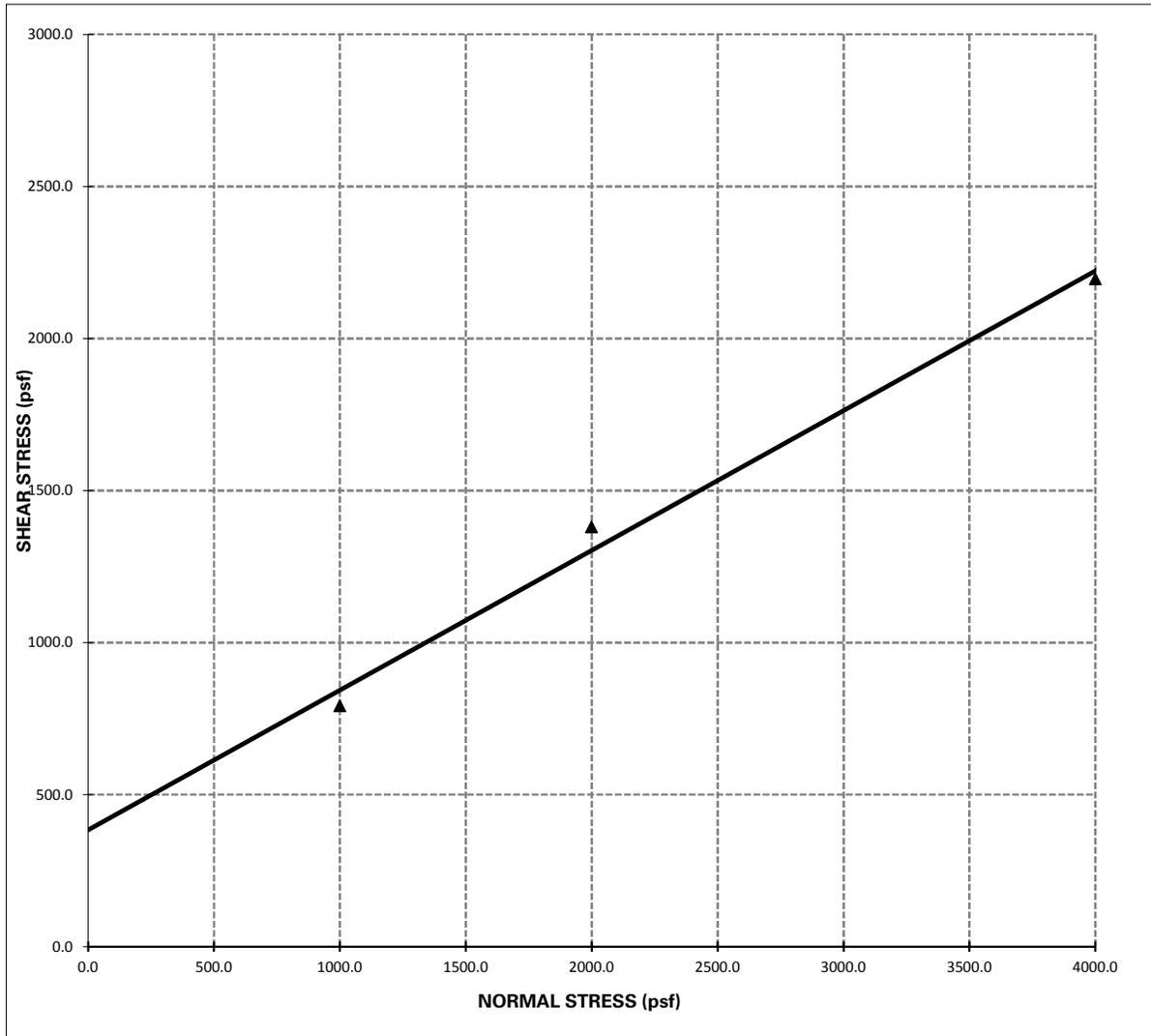
**Shear Strength:**  $\Phi = 24.7^\circ$  ; **C = 384.00 psf**
