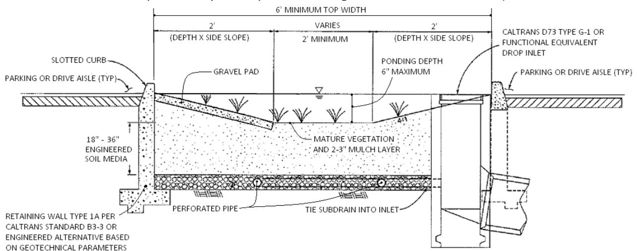
While the 18-inch minimum engineered soil media depth can be used in some cases, it is recommended to use 24 inches or a preferred 36 inches to provide an adequate root zone for the chosen plant palette. Such a design also provides for improved removal effectiveness for nutrients. The recommended ponding depth inside of a Bioretention Facility is 6 inches; measured from the flat bottom surface to the top of the water surface as shown in Figure 1.
