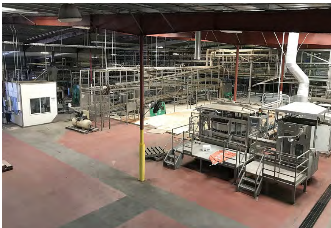
Photo No. 36 Interior of the retail building with filling and canning equipment with associated vats and piping, conveyors, electrical cabinets, a propane tank, and x-ray equipment
