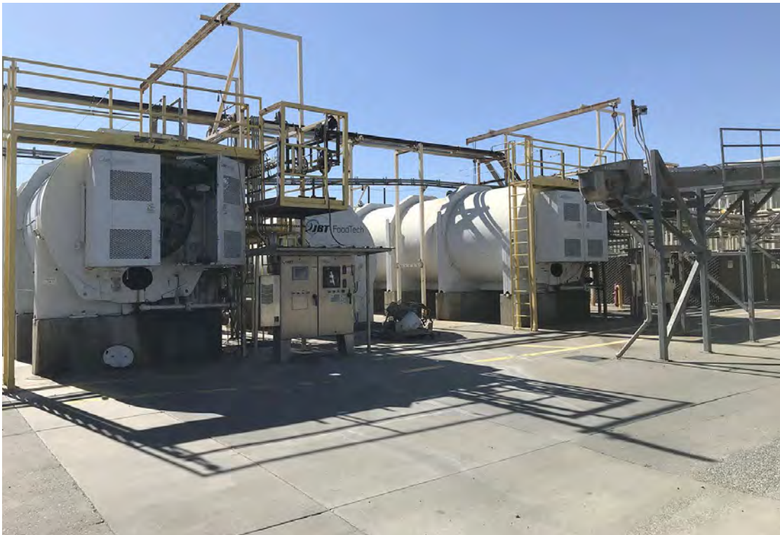
Photo No. 42 View to the southwest of rotary pressure cookers and coolers and conveyor equipment in between the retail building and the south warehouse
