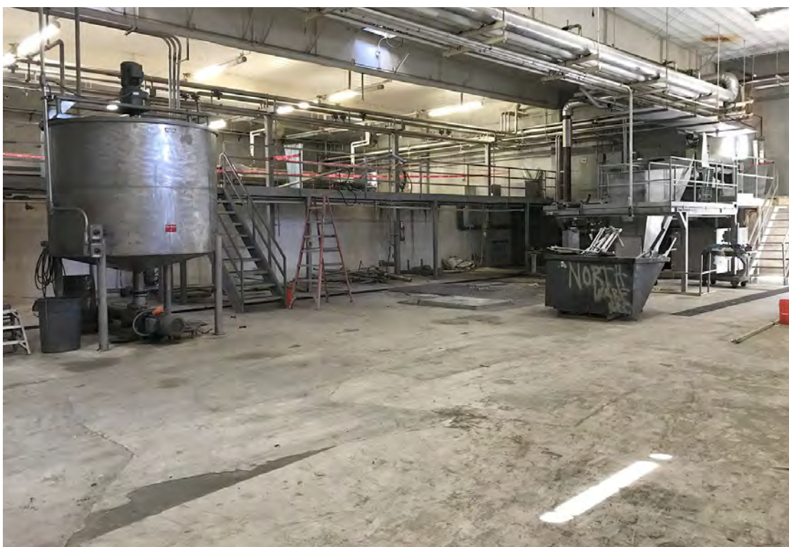
Photo No. 20 Interior of processing room with vats, conveyers, sorting station (upper level), and trench drains
