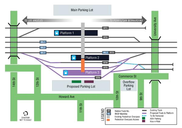
Figure 2-1. Build Alternative Elements
