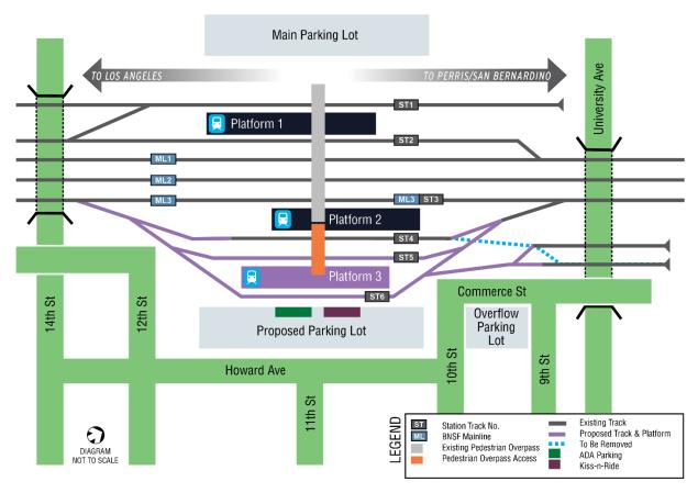
Figure 2-1. Build Alternative Elements
