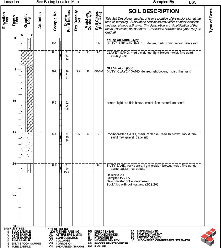
Project No. 2-28-20 12624.001 **Date Drilled Project** RCTC Downtown Station Expansion **BSS** Logged By **Drilling Co.** 2R Drilling **Hole Diameter** 8" **Drilling Method** Hollow Stem Auger - 140lb - Autohammer - 30" Drop **Ground Elevation** NA' Location See Boring Location Map Sampled By
