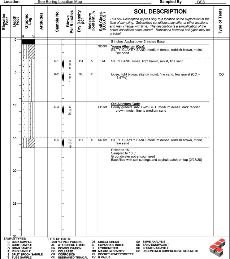
BORING LOCATION (feet): See Plate 2 ELEVATION AND DATUM (feet):
