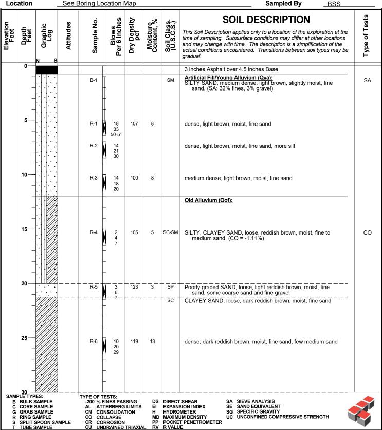
Project No. 2-28-20 12624.001 **Date Drilled Project** RCTC Downtown Station Expansion **BSS** Logged By **Drilling Co.** 2R Drilling **Hole Diameter** 8" **Drilling Method** Hollow Stem Auger - 140lb - Autohammer - 30" Drop **Ground Elevation** NA'
