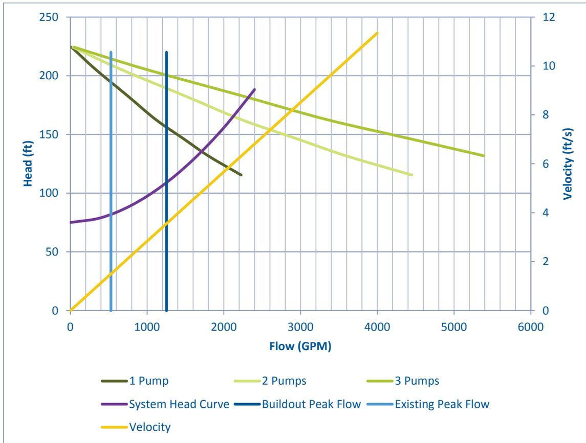
**Figure 5: Day Street Lift Station Capacity Assessment**
