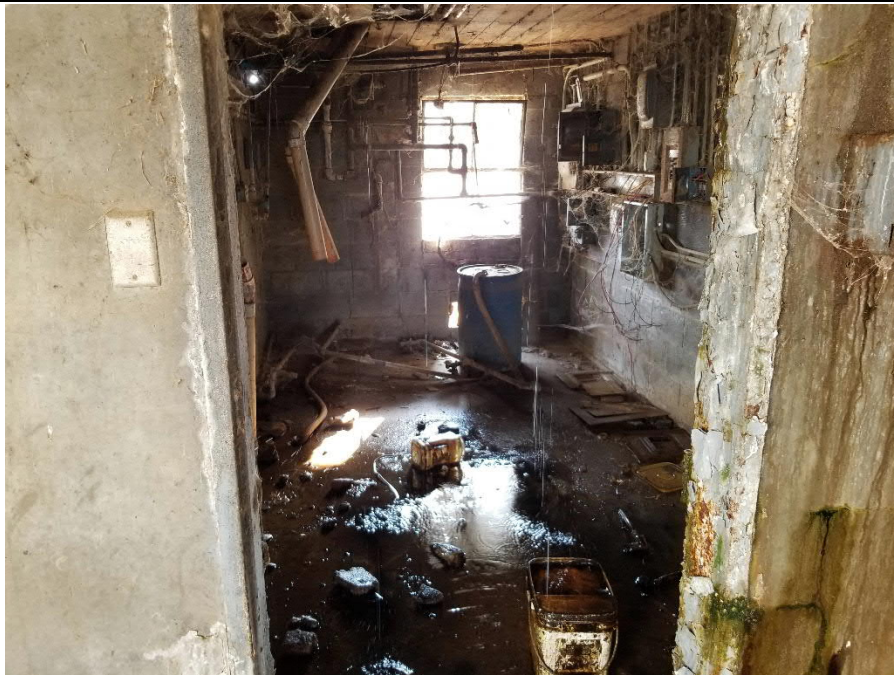
Photo 5: Interior view of abandoned dairy with 55-gallon drum with unknown current volume and contents, and view of surface staining in room that appears to be a petroleum product. BSK did not enter room fully as a safety precaution. The staining and contents within the 55-gallon drum and the room qualify as a REC.
