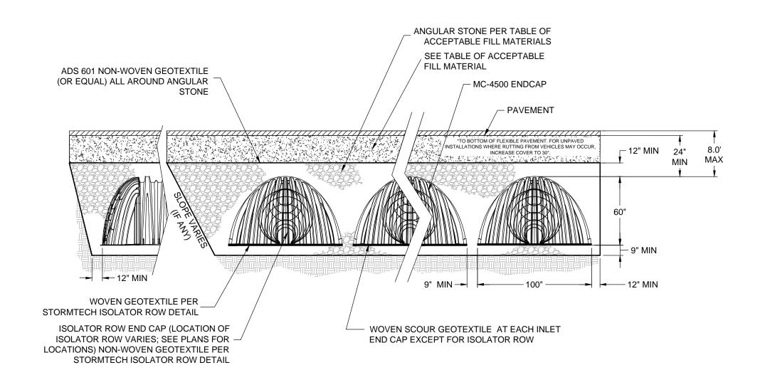
THE INSTALLED CHAMBER SYSTEM SHALL PROVIDE THE LOAD FACTORS SPECIFIED IN THE AASHTO LRFD BRIDGE DESIGN SPECIFICATIONS SECTION 12.12 FOR EARTH AND LIVE LOADS, WITH CONSIDERATION FOR IMPACT AND MULTIPLE VEHICLE PRESENCES.
