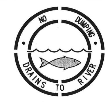
SAMPLE STENCIL TO BE USED NEAR GRATE AND CURB OPENING INLETS SYMBOL TO BE 24" IN DIAMETER
