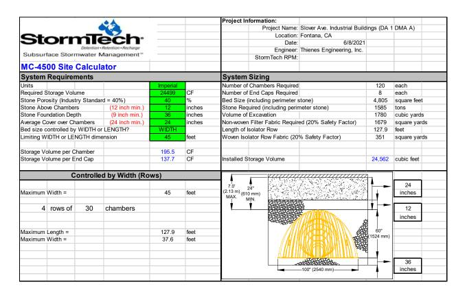
Design infiltration rate = 6.7 in/hr  $d_{max}$  = 160.8 inches = Design infiltration rate x 24 hours = 6.7 in/hr x 24 hrs  $d_{BMP}$  = 79.2 inches = [ (12 inches + 36 inches) x 0.40 ] + 60 inches  $d_{max} > d_{BMP}$
