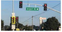
**Bicycle Signals** are used at intersections to separate bicycle movements from conflicting vehicles such as cars, buses, and trolleys. These signals can increase safety and reduce bicyclist and vehicle conflicts.
