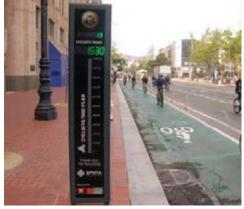
**Automatic Active Transportation Counters** are physical structures that are used to collect bicyclist and pedestrian volumes on a specific corridor. These are intended to remain in place permanently and collect data 24 hours per day, consistent with vehicle counters along roadways. These counters can provide the City with information about pedestrian and bicyclist activity along corridors of interest.
