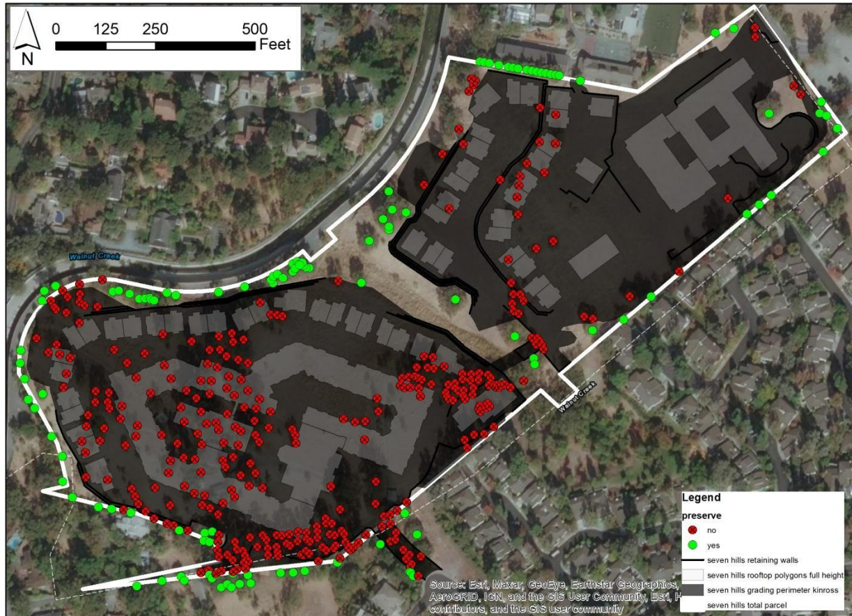
Figure 1. Dark gray area shows the extent of proposed (minimum) grading area. Red dots indicate trees proposed to be cut and green dots indicate trees proposed to be preserved (left uncut but not guaranteed to survive).
