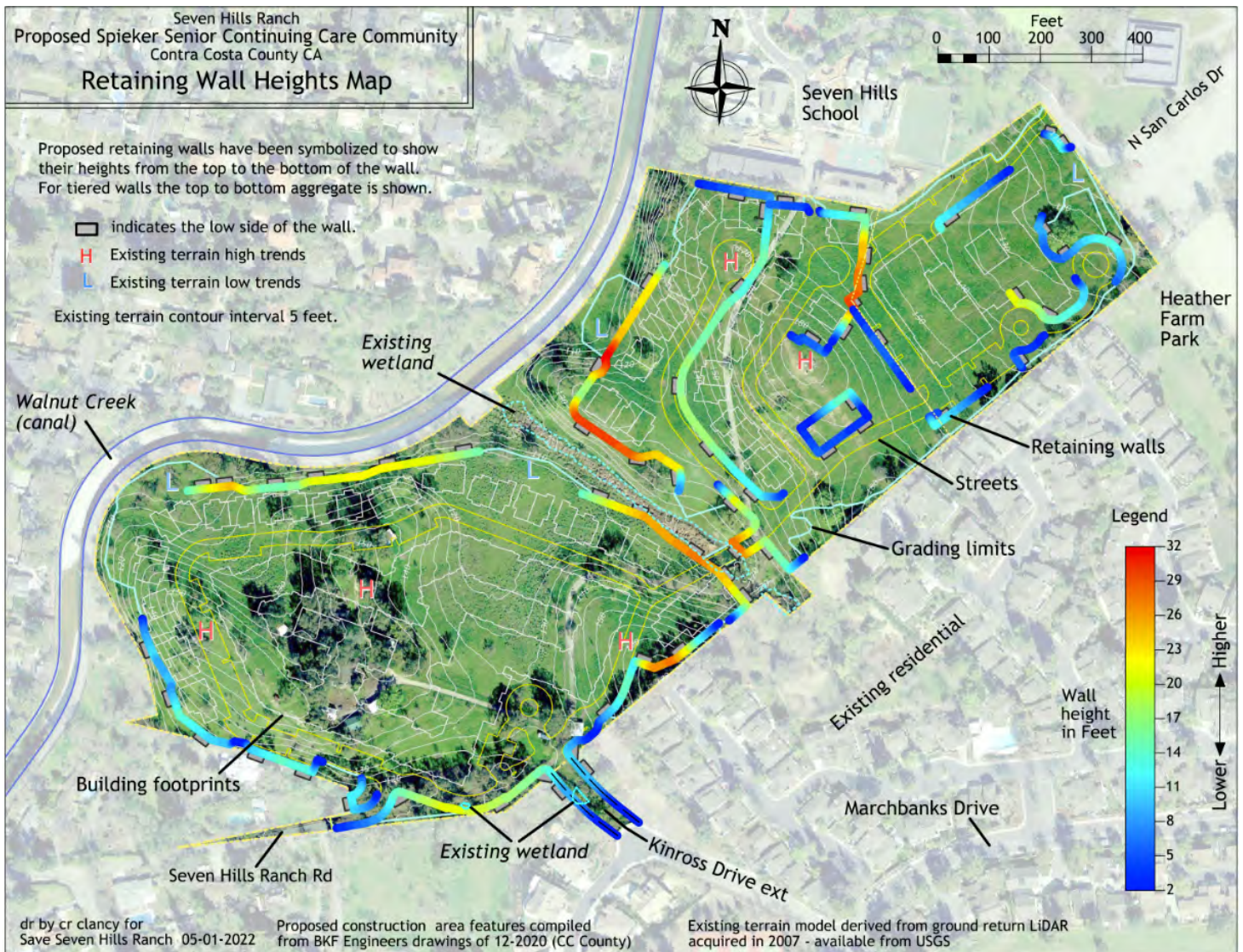
Figure 6 Retaining Walls map. This map indicates the location and color-coded heights of the required retaining walls should the project be allowed to proceed. The higher walls are tiered groupings. 5.1.22
