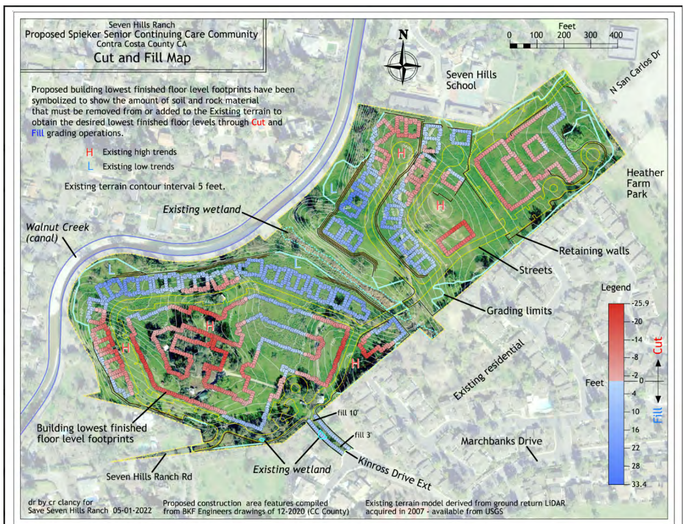
Figure 3 Cut & Fill . This map indicates the extreme amount of grading and landscape altering which will be required should the project be allowed to proceed. With the exception of one, the hills will be leveled. 5.1.22
