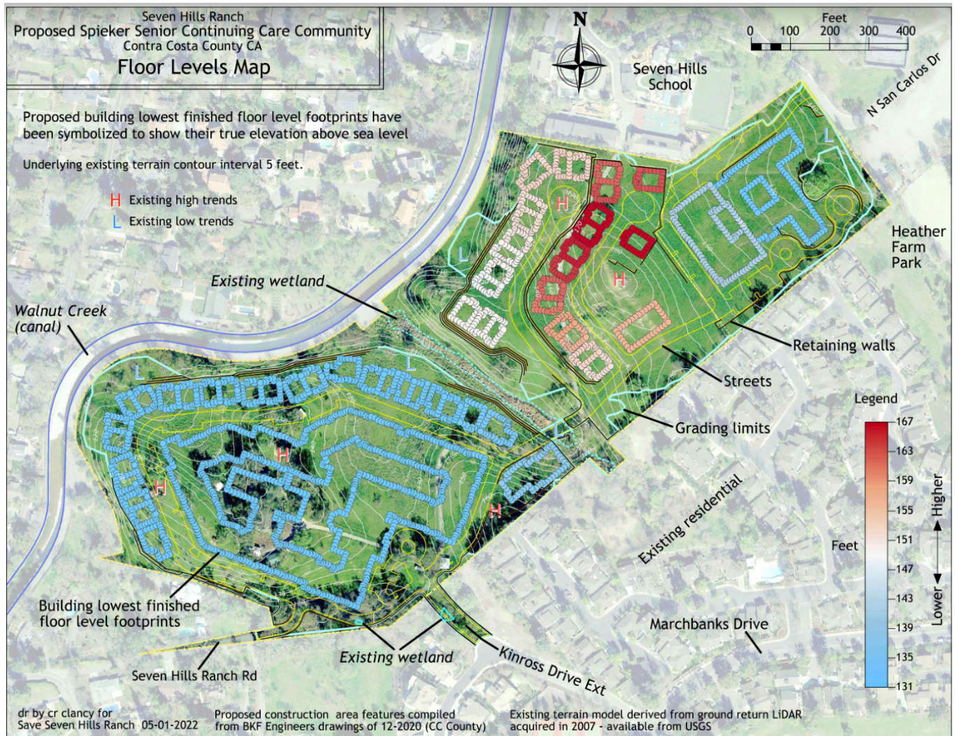
Floor Levels Map - Legend on right, map shows the elevation of the finished floor level.
