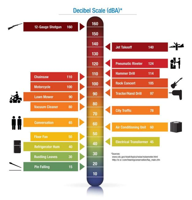
Figure 4 Noise Levels Associated with Common Noise Sources
