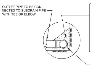
FILTER MATERIAL - MINIMUM OF FIVE CUBIC FEET PER FOOT OF PIPE. SEE ABOVE FOR FILTER MATERIAL SPECIFICATION.
