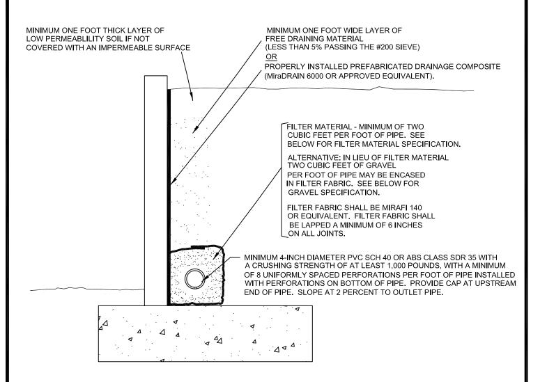
"FILTER MATERIAL" TO MEET FOLLOWING SPECIFICATION OR APPROVED EQUIVALENT: (CONFORMS TO EMA STD. PLAN 323)
