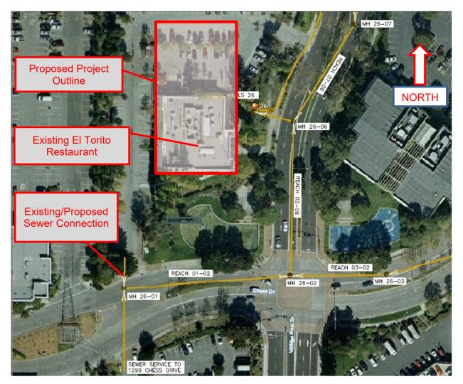
Gravity sewers in the vicinity of the Proposed Project all flow into Lift Station 26, located between the El Torito restaurant and Vintage Park Drive. The Proposed Project will connect to the existing sewer system at Manhole 26-01, located at the end of the southern driveway in Chess Drive. This is the same manhole to which the restaurant is currently connected.
