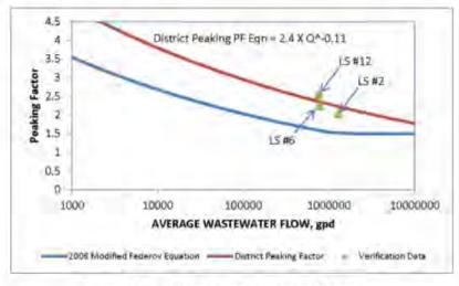
Figure 5-12 Sewer System Peaking Factors
