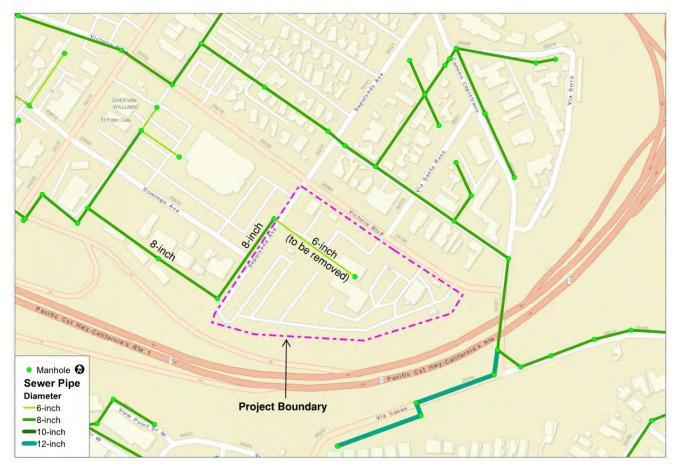
Figure 1-2: Project Location and Existing Sewer System
