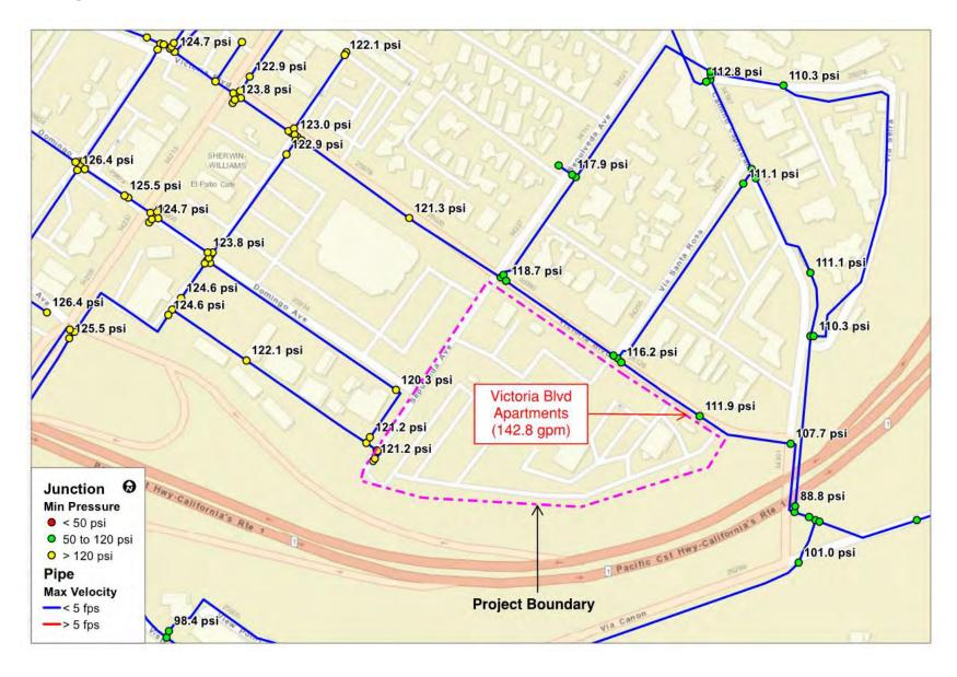
Figure 2-4: Future (2040) MDD with Victoria Blvd Apartments MDD Results Analysis – Minimum Pressures and Maximum Velocities
