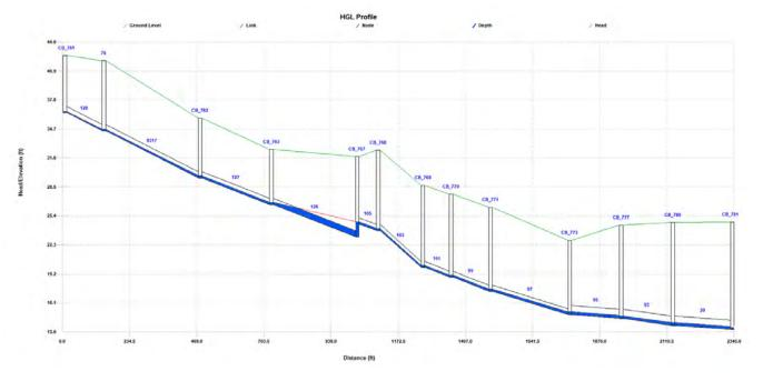
Figure 3-2: Existing Sewer Model Pipe Profile at Alley South of Domingo Ave and Doheny Park Rd
