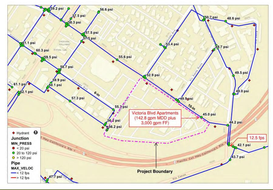
Figure 2-5: Run 1 - Future (2040) MDD with Victoria Blvd Apartments MDD plus FF Results Analysis – Minimum Pressures and Maximum Velocities
