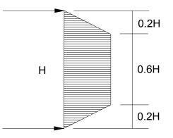
7.17.19 Where a combination of sloped embankment and shoring is utilized, the pressure will be greater and must be determined for each combination. Additional active pressure should be added for a surcharge condition due to sloping ground, vehicular traffic, or adjacent structures and must be determined for each combination.
